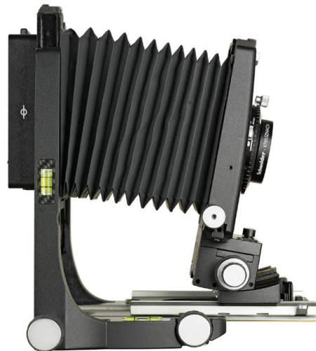
Vertical shift at the rear standard and tilting of the lens standard for Scheimpflug rule.
