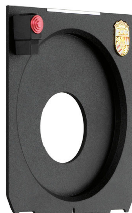
Recessed Technika 45 Lensboard with Cable Release Socket and cutout for Copal 0, 6 mm recessed. 001047
