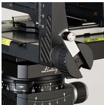
Fast wind lever for rear standard at Linhof Techno. Larger shifts can now be realized faster. 002770
