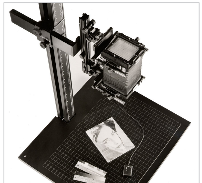
TECHNOPRO II Solid repro column as desk device or with special steel table. For medium format or large format cameras with film or digital back. Illustration: Linhof RD 1 (000140) with Compendium (001934) on Technopro II (003015), below with 4x5 camera.
